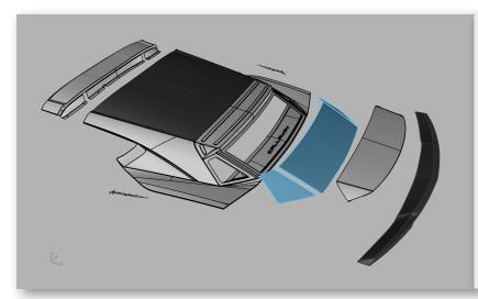
The AeroWagen package is supplied as ready to bolt on, single piece carbon fiber molding. No fabrication is required. Paint to match options are detailed at the website. The standard hatch can be re-installed.
