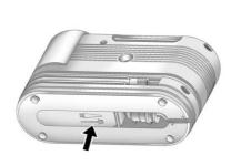
The tire sealant and compressor kit has an accessory adapter located in a compartment on the bottom of its housing that may be used to inflate air mattresses, balls, etc.
