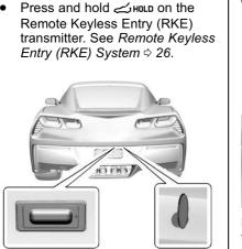
Press the hatch/trunk release touch pad with the RKE transmitter within range or use the key in the key cylinder. See *Remote Keyless Entry (RKE) System* ⇔ 26 and Keys ⇔ 25.
