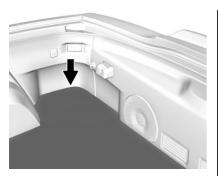
4. Open the rear hatch/trunk and lift the carpet on the passenger side of the vehicle to gain access to the battery cover.
