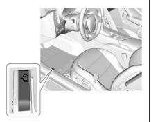
From inside the vehicle, pull the door release handle.
