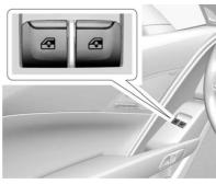
Pull up or press down on the switch to raise or lower the window. See *Power Windows* ⇔ 45.
