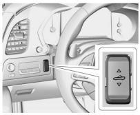
Press and hold the bottom of عنه. The windows will automatically lower.  After the convertible top is completely open, a chime sounds and a DIC message displays. Release the switch.
