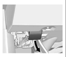
1. Pull the hood release lever inside the vehicle. It is below the instrument panel on the driver side.
