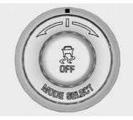
The PTM system contains five modes. These modes are selected by turning the Selective Ride Control/Performance Traction Management MODE SELECT knob on the center console. Scroll up or down through modes 1–5 by turning the MODE SELECT knob to the right or left.
