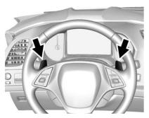
The Manual Paddle Shift system can be used in D (Drive) or M (Manual Mode). The system is activated by pushing the left paddle to downshift and the right paddle to upshift. The current gear will be displayed in the instrument cluster, or the Head-Up Display (HUD), if equipped. The Manual Paddle Shift system will not allow either an upshift or a downshift if the vehicle speed is too fast or too slow, nor will it allow a start from 3 (Third) or higher gear.
