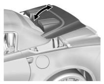
1. On each side of the tonneau cover, lift and pivot rearward into the fully open position.
