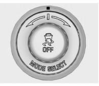
In order to select this optional handling mode, the vehicle mode must be Track. Then quickly press the TCS/StabiliTrak 🛱 button on the center console two times. STABILITRAK COMPETITIVE MODE displays in the Driver Information Center (DIC). See *Ride Control System Messages* ⇔ 125.
