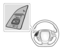
$\infty$  (On/Off) : Press to turn cruise control on or off. A white indicator comes on in the instrument cluster when cruise is turned on.
