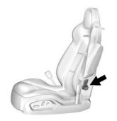
If equipped, lift the latch to fold a seatback forward.
