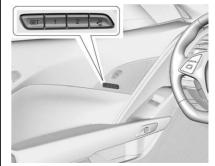
If equipped, the 1, 2, SET, and 1 (Exit) buttons on the driver door are used to manually store and recall memory settings for the driver seat, outside mirrors, and power tilt and telescoping steering column.
