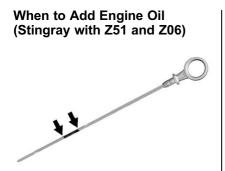
If the oil is below the cross-hatched area at the tip of the dipstick, add 1 L (1 qt) of the recommended oil through the oil fill cap opening in the oil tank and then recheck the level. See "Selecting the Right Engine Oil" for an explanation of what kind of oil to use. For engine oil crankcase capacity, see *Capacities and Specifications*  $\Rightarrow$  312.
