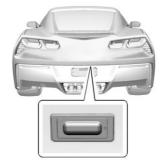
Press the release touch pad to open the trunk if the RKE transmitter is within 1 m (3 ft).
