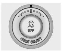
The TCS/StabiliTrak button is on the center console.
