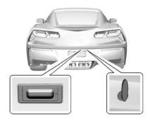
Press the hatch/trunk release touch pad with the RKE transmitter within range or use the key in the key cylinder. See *Keys*  $\Rightarrow$  25.
