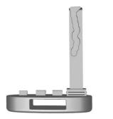
The key inside the RKE transmitter can be used to open the vehicle and hatch/trunk if power to the vehicle is lost. See *Hatch (Trunk)*  $\Rightarrow$  37.
