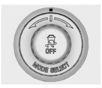
The Driver Mode Selector knob is on the console behind the shift lever.
