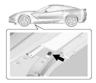
Use only a service jack with a lifting pad diameter of 64 mm (2.5 in) or smaller, and thick enough to make sure the jack does not contact the vehicle body.
