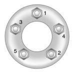
Tighten the wheel lug nuts firmly in a crisscross sequence. See *Capacities and Specifications* ⇔ 312.
