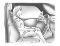
If a person of adult size is sitting in the front outboard passenger seat, but the off indicator is lit, it could be because that person is not sitting properly in the seat or that the child restraint locking feature is engaged. Use the following steps to allow the system to detect that person and enable the front outboard passenger frontal airbag:
