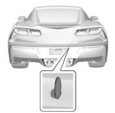
From outside the vehicle, use the key to open the hatch/trunk. See *Keys*  $\Leftrightarrow$  25.
