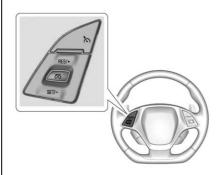
S: Press to turn cruise control on or off. A white indicator comes on in the instrument cluster when cruise is turned on.
