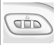
This system, if equipped, provides a way to replace up to three remote control transmitters used to activate devices such as garage door openers, security systems, and home automation devices.
