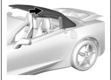
2. Lift and pivot the convertible top rearward into the fully stowed position.
