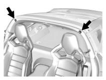
Position the rear edge of the roof panel next to the weatherstrip on the back of the roof opening. Then align and fit the pins at the rear of the roof panel inside the openings in the rear overhead weatherstrip. Gently lower the front edge of the roof panel to the front of the roof opening.
