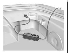
Some vehicles have a battery maintainer package. Follow the instructions provided with the battery maintainer package to keep the battery charged when the vehicle is not in use. Plug the battery maintainer into the rear accessory power outlet only. The front APO turns off after the ignition is off.
