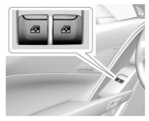
Press the switch to the first detent to lower the window. Pull to the first detent to raise the window. Release to stop at the desired position.
