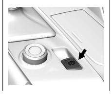
The vehicle has an Electric Parking Brake (EPB). The switch is on the center console. The EPB can always be activated, even if the ignition is off. To prevent draining the battery, avoid repeated cycles of the EPB when the engine is not running.
