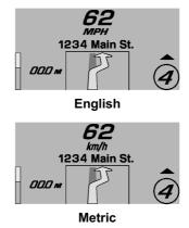
**Navigation :** Turn-by-turn navigation information may be displayed when Navigation is active and an upcoming maneuver is pending. It appears until the maneuver is complete and then the HUD display returns to the previous view.
