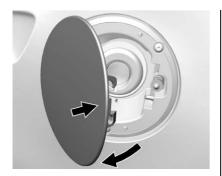
To open the fuel door, push and release the rearward center edge of the door. The fuel door is locked when the vehicle doors are locked. Press and on the RKE transmitter to unlock. The driver door must be opened before the fuel door will unlock.
