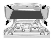
Attach the elastic loops on the four corners of the cargo cover to the hooks on the front and rear corners of the hatch.
